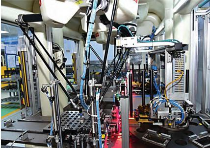
A high-on-automation manufacturing setup at Gabriel India's facility in Hosur, Tamil Nadu. The company has implemented automation at the valving stage during a damper's production.
