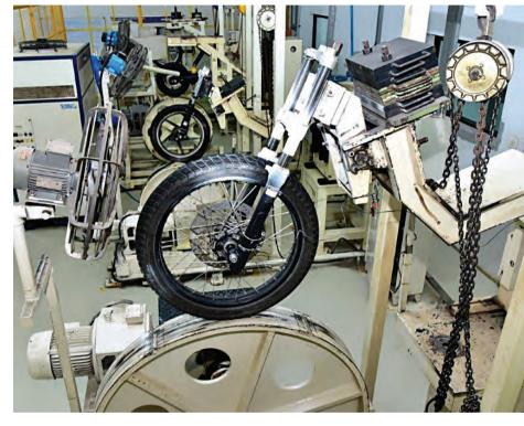
From L to R: Suspension systems being jig tested at Gabriel India's two-wheeler development and test facility in Hosur, while its four-wheeler engineering centre in Chakan is replete with sophisticated test equipment including motion simulators.
